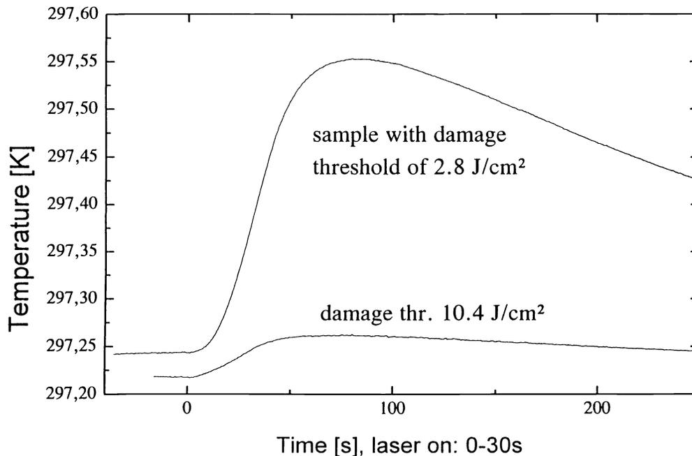
Fig. 2: Temperature vs. time curves for two laser irradiated HR coatings deposited under normal and high purity conditions, respectively; laser parameters: wavelength 248nm, pulse length 30ns, repetition rate 150Hz, pulse energy density 175mJ/cm<sup>2</sup>; respective damage thresholds are shown
