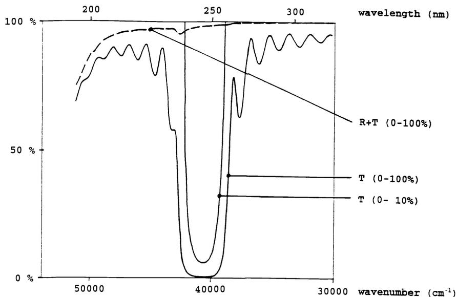
Fig. 1: Transmittance and transmittance + reflectance spectrum of a high purity Al<sub>2</sub>O<sub>3</sub>/SiO<sub>2</sub> HR coating S | (HL)<sup>20</sup>HLL | Air
