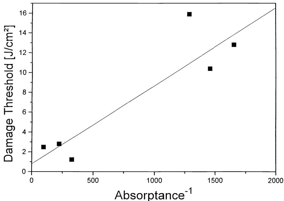
Fig. 3: Damage thresholds vs. inverse of absorptance, laser parameters as in Fig. 2
