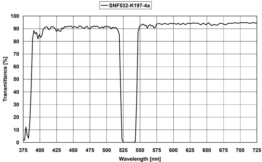
**Figure 8:** Measured spectral notch filter performance, SNF532OD5
