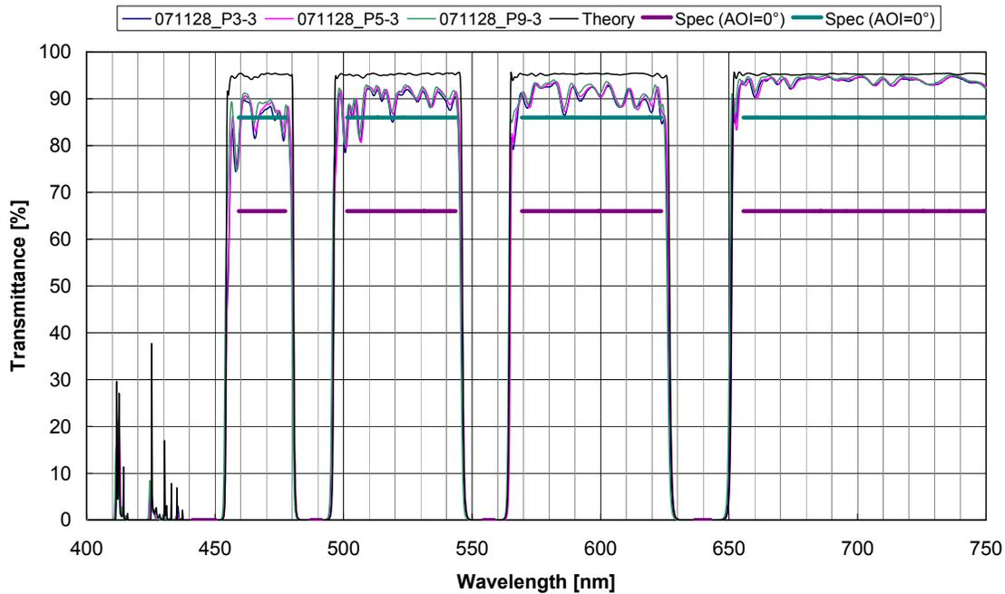
**Figure 13:** Spectral performance in transmittance of a quadruple multi notch filter based on Nb<sub>2</sub>O<sub>5</sub> / SiO<sub>2</sub> for AOI 0°.
