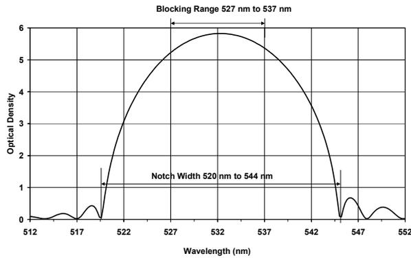
Figure 3: Notch filter characteristic with  $\rho=1.072$  and  $s=106$ .
