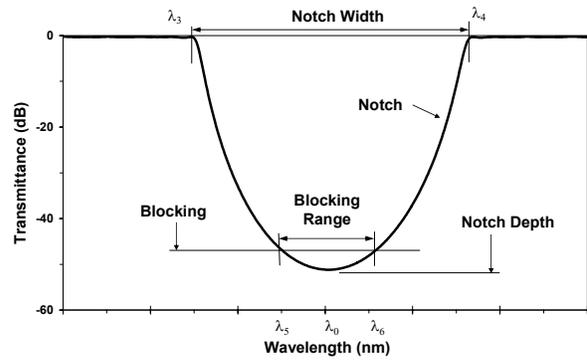
**Figure 2:** Definition of a notch filter characteristic
