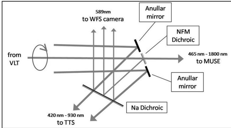
**Figure 2:** Scheme of the beam paths at the dichroics of the GALACSI optics.
