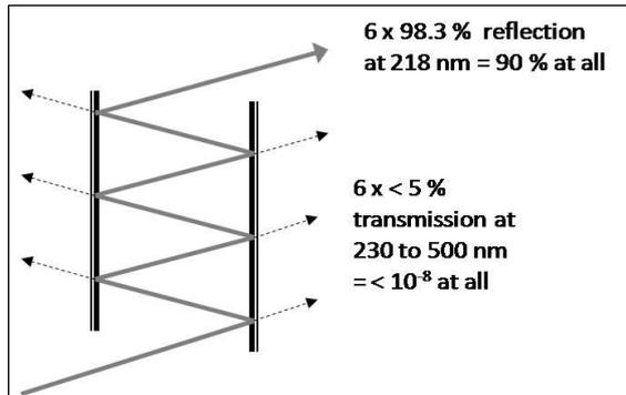
**Figure 12:** Schematic optical design with 6 reflections at 15 degrees AOI between two parallel plates deposited with the 218nm NF (see text).
