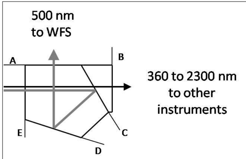
**Figure 10:** Schematic of the optical design of the 500nm beam splitter, the lines with the capitals A to E mark the different faces at the prism group (see the text).
