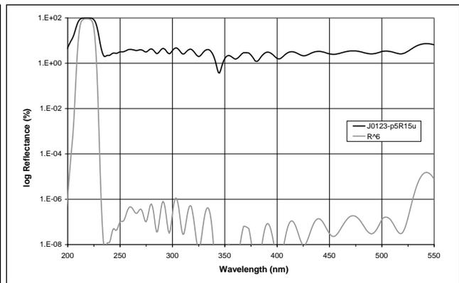
**Figure 13a (left):** 218nm NF measured in reflectance at a single plate. **Figure 13b (right):** 218nm NF reflectance in logarithm scale, at a single plate and after 6 reflections inside the two reflection plates.
