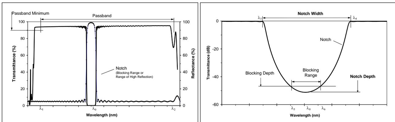
**Figure 5a (left):** Single NF characteristic with the parameters passband, passband minimum, and blocking range. **Figure 5b (right):** NF characteristic with the definition of the parameters notch width, notch depth, blocking range, and blocking depth.
