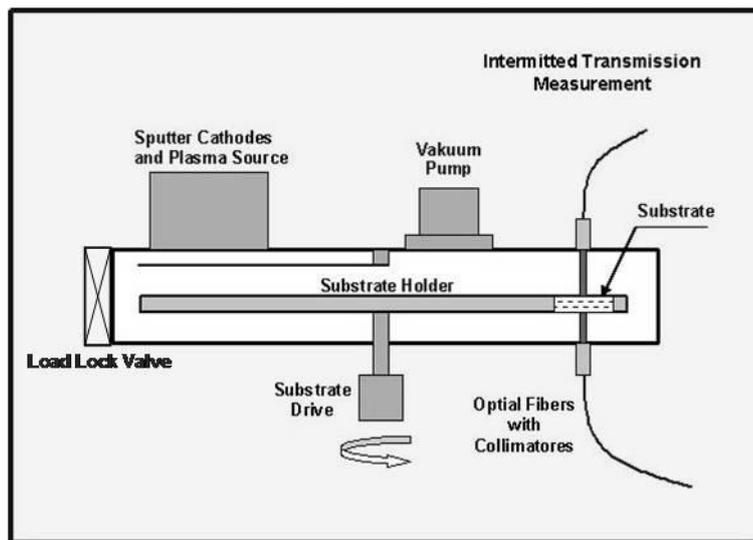
**Figure 7:** Principle of the PARMs technology and the broadband wavelength intermittent monitoring at the HELIOS sputtering tool (courtesy of Leybold Optics).
