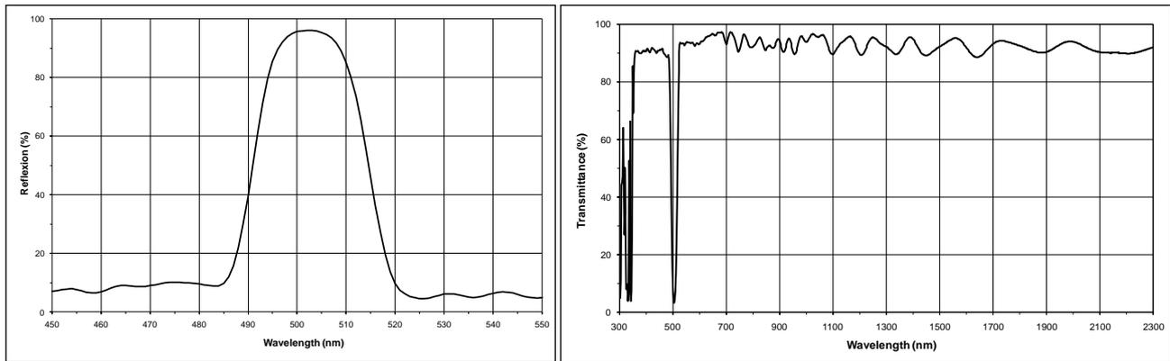
**Figure 11a (left):** 500nm beam splitter measured in transmittance through the complete prism-group. **Figure 11b (right):** 500nm beam splitter measured in reflection at a witness sample.
