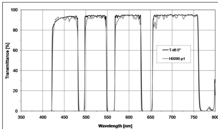
**Figure 14:** Comparison of measured (H0090-p1) and specified transmittance (T-d6 0°) of the multi NF based on Ta<sub>2</sub>O<sub>5</sub> / SiO<sub>2</sub> for AOI 0°. In all four notches or reflectance bands the blocking range is better than OD4.
