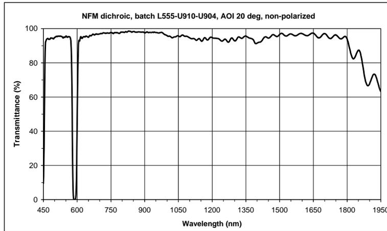
**Figure 4:** NFM dichroic of the GALCXI optics measured in transmission at 20 degrees AOI, non-polarised.
