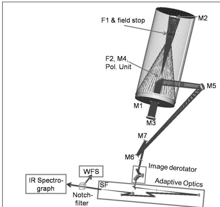
**Figure 8:** The optical design of the GREGOR telescope with a notch filter at the end of the optical path as a first beam splitter (courtesy of KIS).
