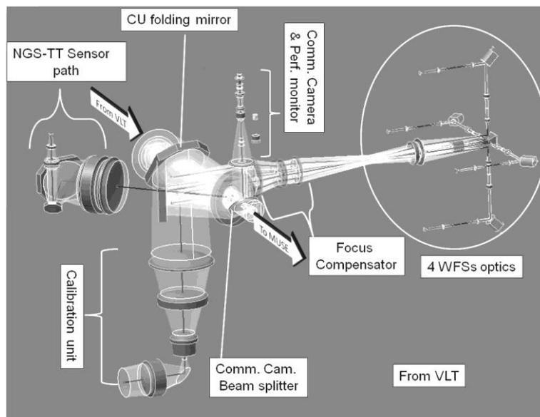
**Figure 1:** Illustration of the optics foreseen for the GALACSI AOF (courtesy of ESO).
