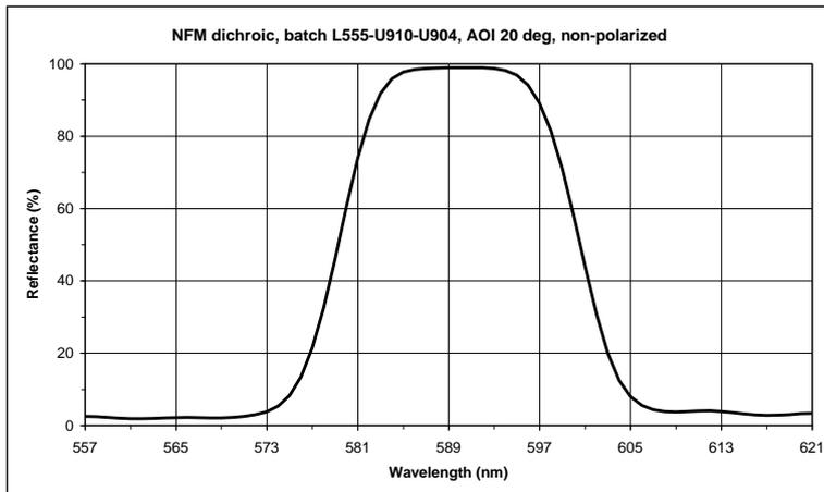
**Figure 3:** NFM dichroic of the GALCXI optics measured in reflection at 20 degrees AOI, non-polarised.
