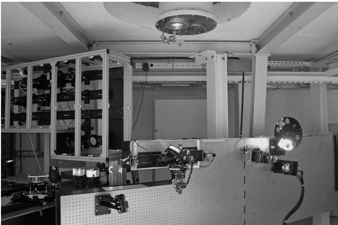
**Figure 9:** The instrument room of the GREGOR telescope with the beam splitters at bottom left (courtesy of KIS).
