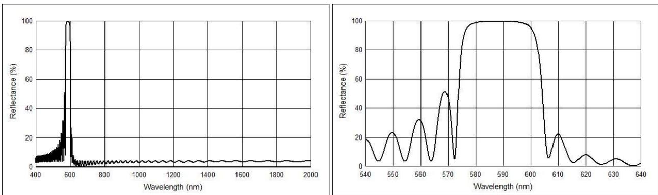
**Figure 6a (left):** Calculated NF transmittance characteristic with a simple  $(8H 195L)^{50}$  layer sequence, **Figure 6b (right):** Calculated notch filter reflectance characteristic as with Figure 6a (see text).
