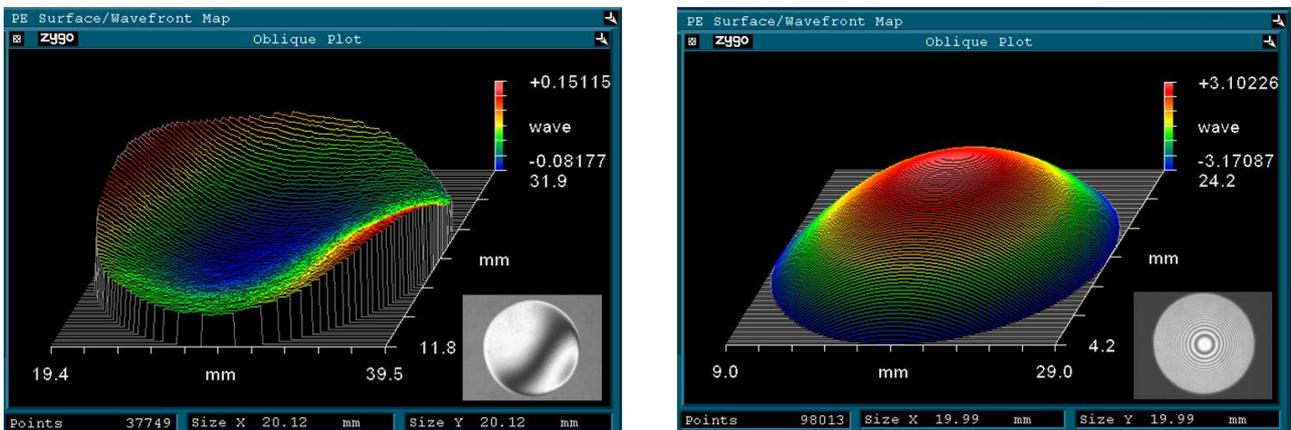
Figure 4. Measured surface deformation of a Ø25mm BK7-test-substrate before (left) and after depositing the 19µm NIR-band-pass-filter (right). The small in-sets show the according interferograms.
