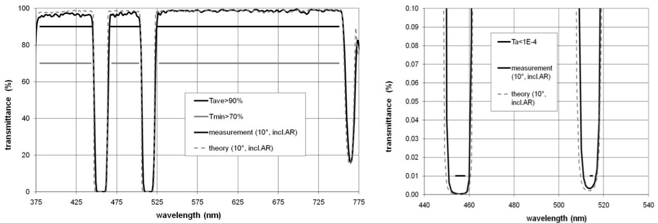
Figure 5. Transmittance (left) and enlargement of the rejection bands (right) of the double-notch-filter.
