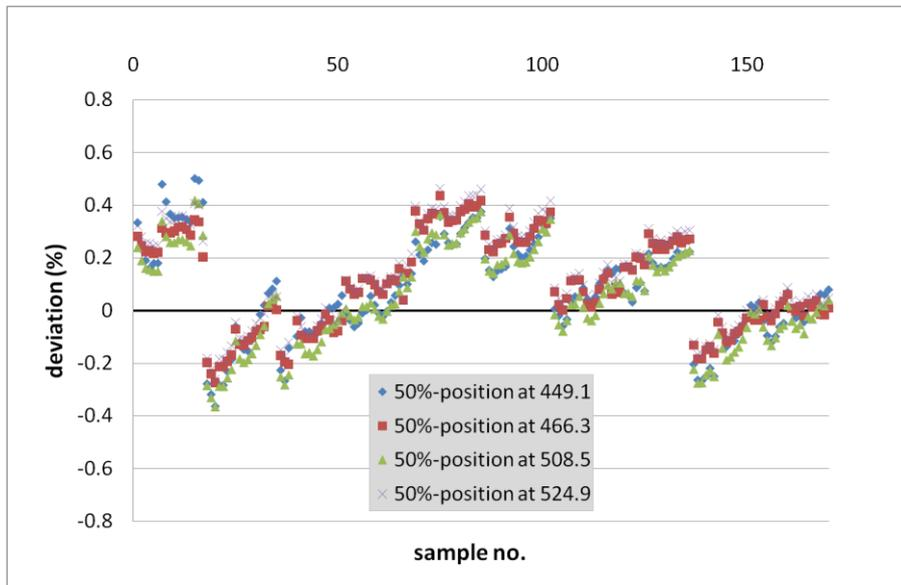
Figure 6. Batch-uniformity calculated at the 50% transmittance values at the 4 edges of the double-notch-filter with respect to the spectral target positions.
