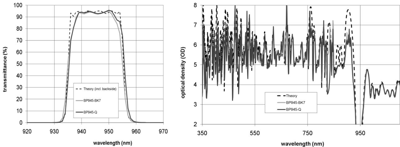
Figure 1. Transmittance (left) and optical density spectra (right) of the NIR-band-pass-filter, including backside reflection. Comparison of measured filters on BK7 and on quartz-substrates with the theoretical values.
