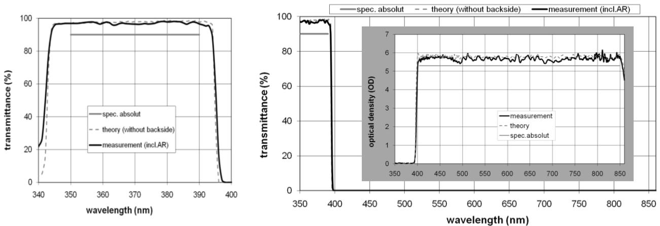
Figure 7. Pass band transmittance (left) and transmittance of the blocking range with optical density (right) of the shortwave pass filter on a quartz substrate.
