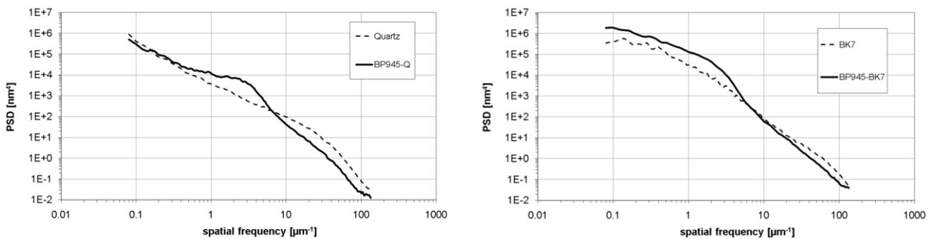
Figure 2. PSD-functions computed from AFM-data of NIR-band-pass-filters and their corresponding substrates, quartz (left) and BK7 (right).
