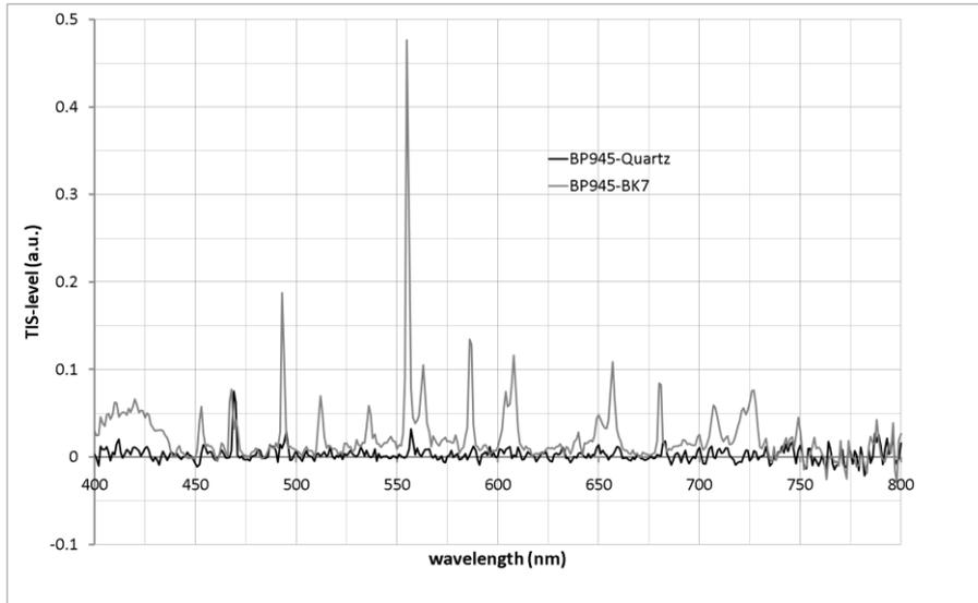
Figure 3. TIS-measurements of two NIR-band-pass-filters on BK7 and quartz-substrates.
