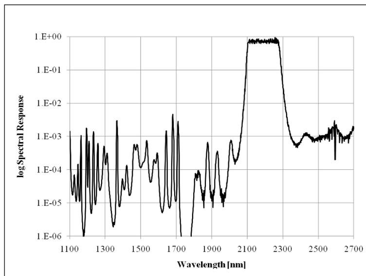
Figure 6. Measured log spectral response for BP2190 integrated response 0.42%
