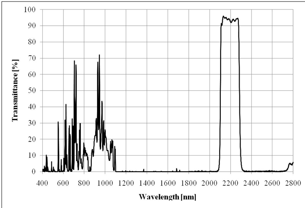
Figure 4. Spectral characteristic of SWIR BP2190 with blocking range from 1100 nm to 2700 nm and monitoring range from 420 nm to 1020 nm
