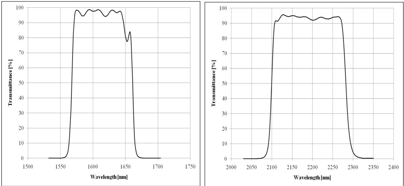
Figure 5. Measured spectral characteristics of BP1610 and BP2190, deviated CWL 1611.1 and 2190.9nm, deviated BW 93.5 and 183.1nm
