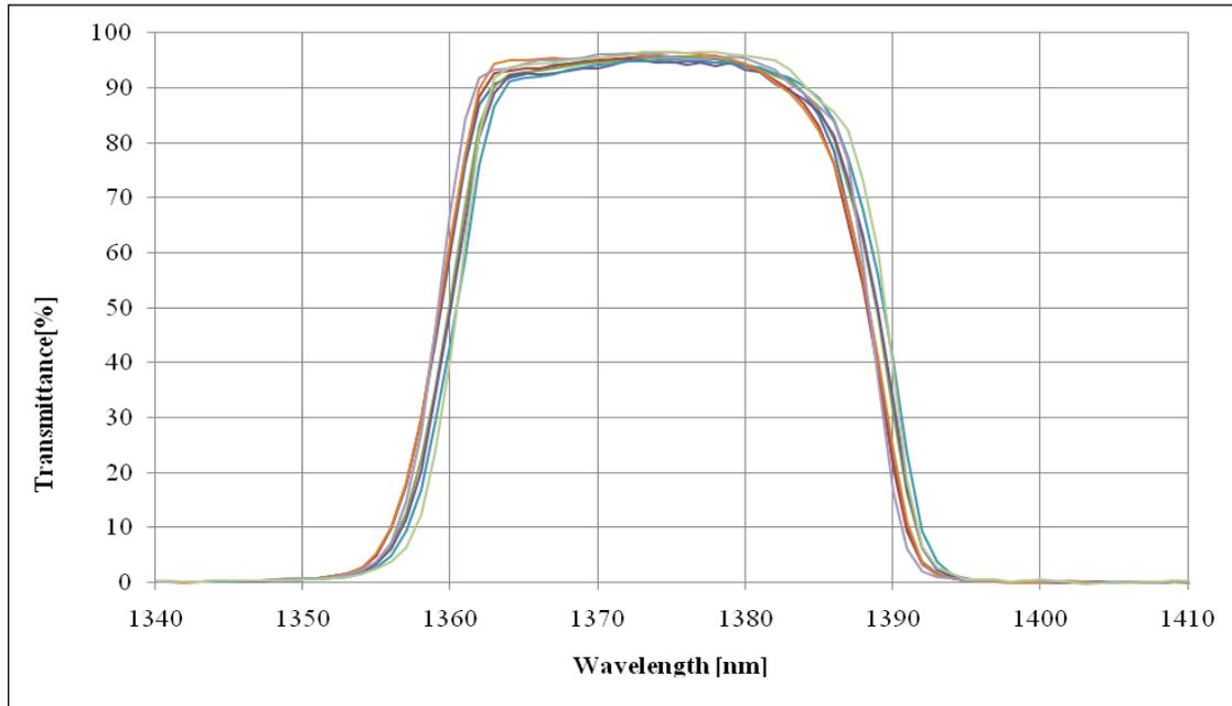
Figure 7. Measured transmittance of 10 BP1375 filters centre wavelength =  $1374.5 \pm 1.2$  nm, bandwidth =  $29.2 \pm 0.8$  nm
