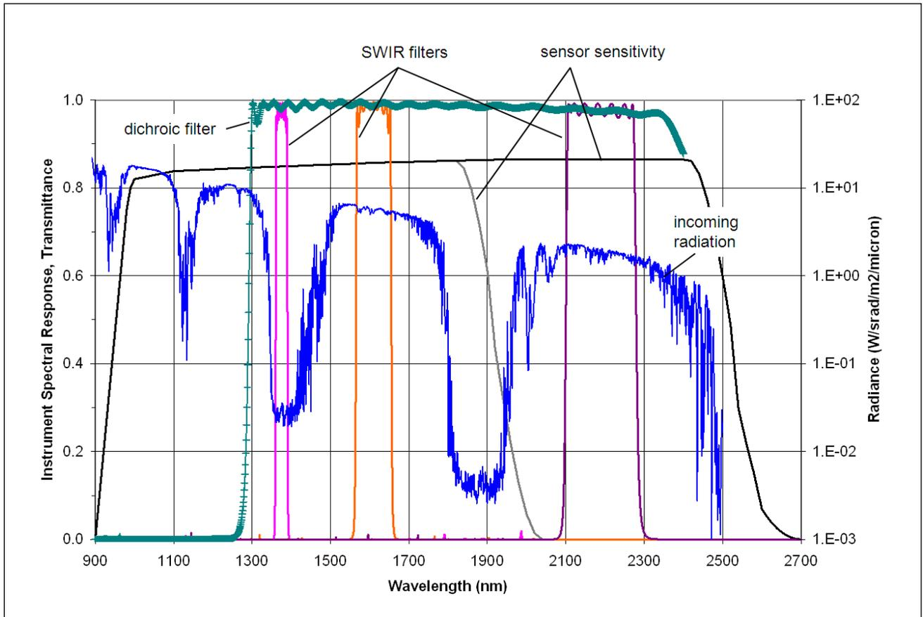
Figure 1. Components of spectral characteristics of SWIR filters: Band-pass filters at 1375 nm, 1610 nm, 2190 nm, incoming radiation, detector sensitivity and dichroic filter (+)
