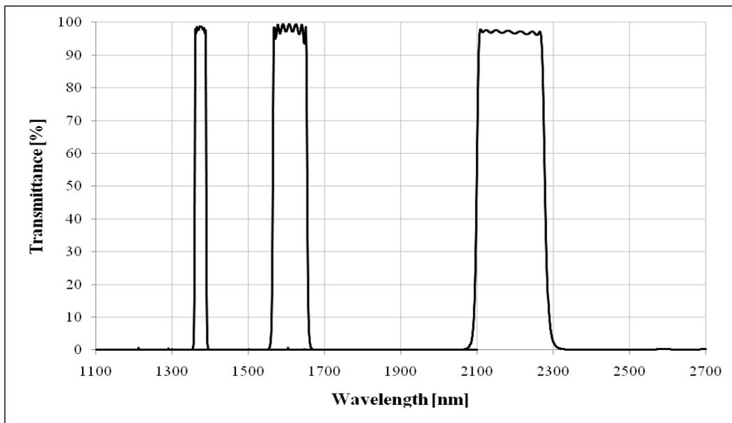
Figure 2. theoretical performance values as a transmittance versus wavelength plot of BP1375, BP 1610 and BP2190
