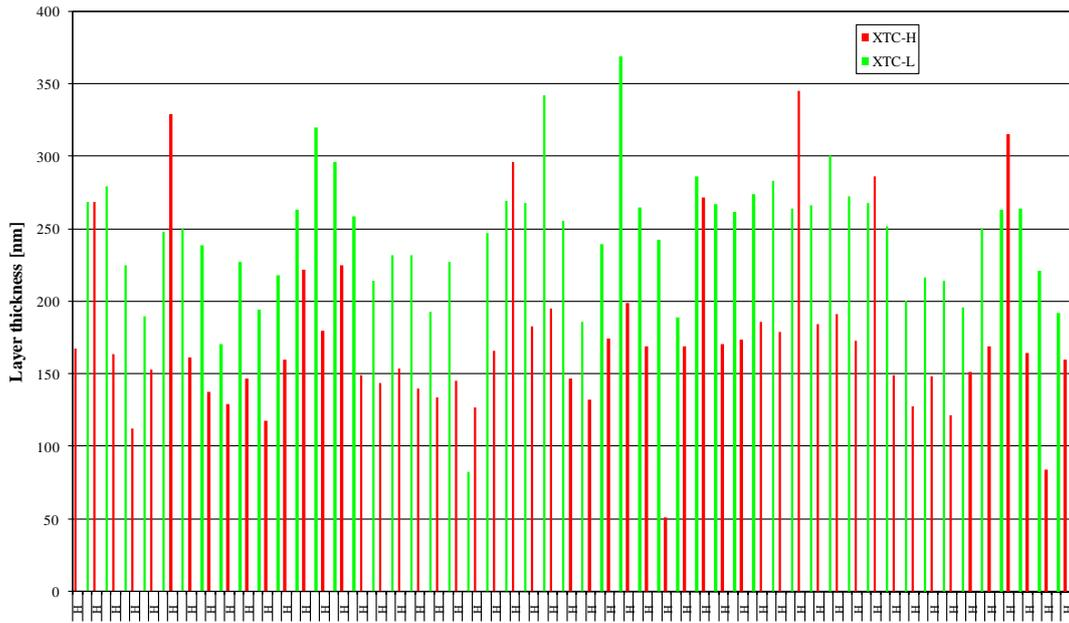
Figure 3. Thickness distribution example: BP1375 with 105 layers, overall physical thickness 22 $\mu$ m, single layer thickness as minimum 51nm, as maximum 366nm
