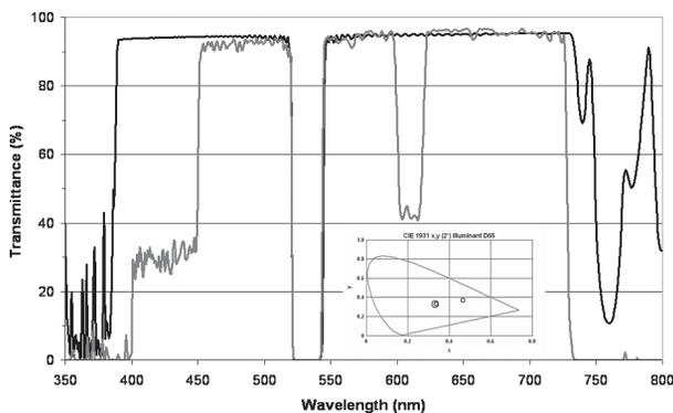
Figure 2: Transmittance of a color-corrected 532nm Notch-filter (grey) with  $x,y$ -color-coordinates  $x = 0.33$  and  $y = 0.33$  (double-circle within the embedded diagram), and an uncorrected 532 nm Notch filter (black) with  $x,y$ -color coordinates  $x = 0.46$  and  $y = 0.36$  (single circle within the embedded diagram).
