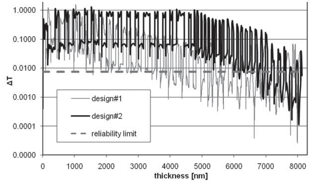
Figure 3: Monitoring  $\Delta T$ -function of two different  $\text{TiO}_2/\text{SiO}_2$  non-quarterwave designs, each with a total thickness of  $8.5 \mu\text{m}$ , in comparison with the reliability limit of the  $\Delta T$ -function, which indicates a necessary change of the monitoring chip [14].
